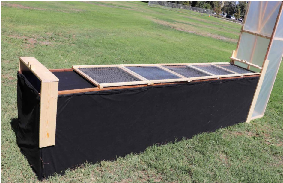
A chimney solar dryer ready for drying fruits and vegetables. Leave the first tray space (left side of photo) empty as a “preheat area.”
