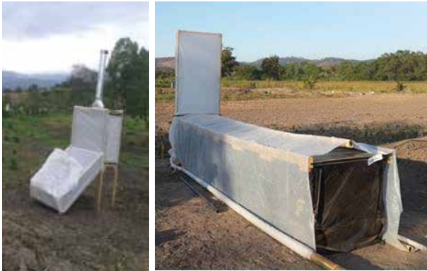
Secadores Solares (Izq. Cabinet Dryer, Der. UCD Dryer)
