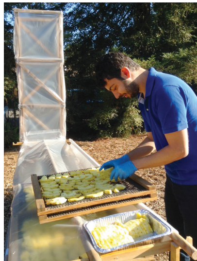
Designed by UC Davis researchers for the Horticulture Innovation Lab, the chimney solar dryer combines solar heat collection with rapid air flow for efficient drying of fresh produce.
