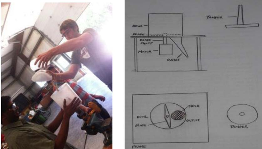
Fig. 1 An illustration of the first prototype and its test set up. The tamper held by the user and placed in the bowl to force grass down towards the blades.
