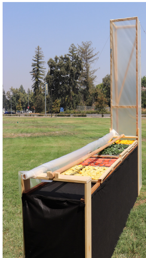
Built with widely available materials, the chimney solar dryer combines a table for drying fruits and vegetables with a chimney.
