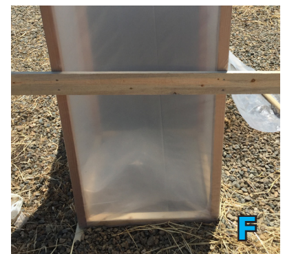
Above: securing the clear plastic covering to one side can help reduce tears. Top right: drip tape placed along edges with staples reduces rips at staple points. Bottom right: a piece of wood secured at the back of the chimney can be used to help with moving the chimney solar dryer if necessary.
