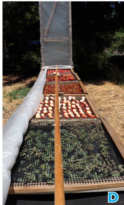
Above: securing the clear plastic covering to one side can help reduce tears. Top right: drip tape placed along edges with staples reduces rips at staple points. Bottom right: a piece of wood secured at the back of the chimney can be used to help with moving the chimney solar dryer if necessary.
