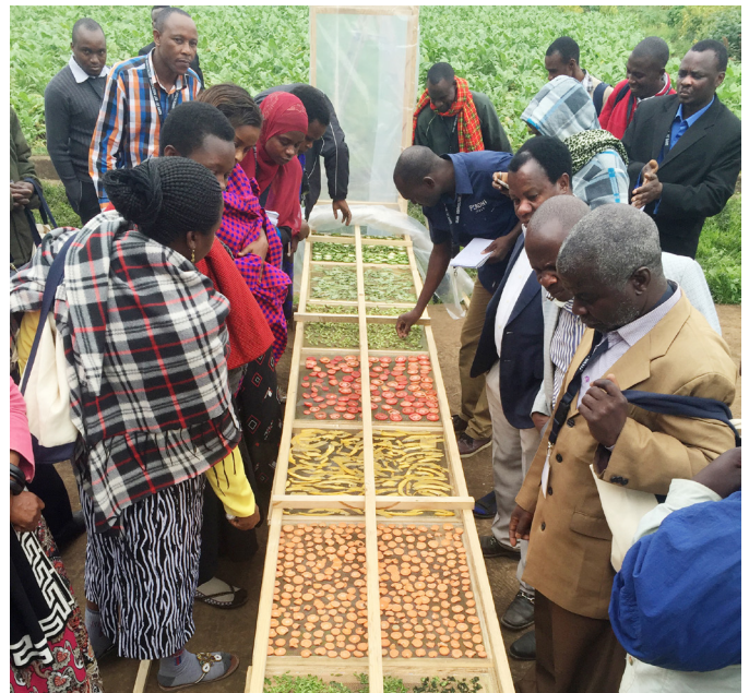
The Horticulture Innovation Lab team has built chimney solar dryers in several countries, including Bangladesh (top photo) and Tanzania (above). Materials and dimensions can be adjusted based on location. (Horticulture Innovation Lab photos by Britta Hansen and Angelos Deltsidis)
