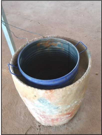
Above are images of clay pot coolers with a metal container in a clay pot configuration at various locations in Rwanda.
