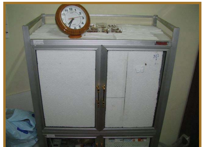
A small aluminum kitchen cabinet (122 cm tall, 77 cm wide, and 41 cm deep) transformed into a seed germinating cabinet
