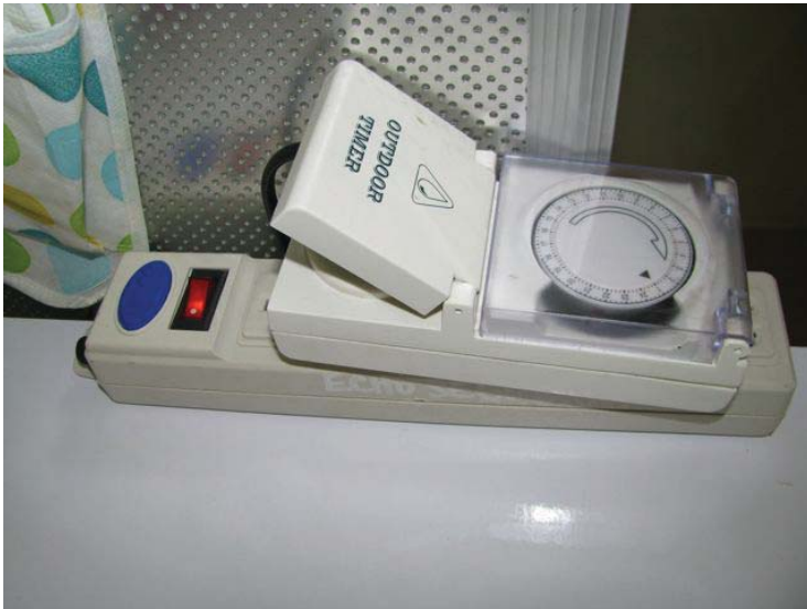
Figure 6: Timer assembly (connected to power strip in figure 5) to regulate florescent tube on/off duration.
