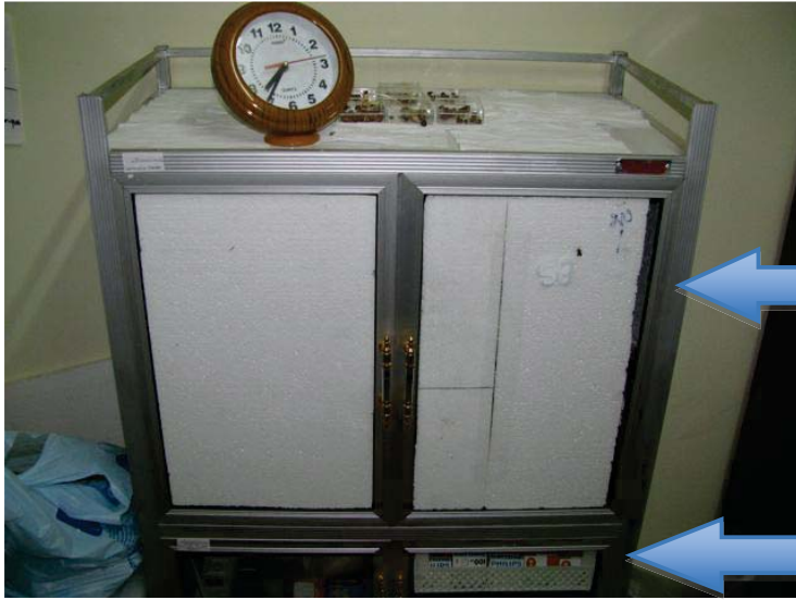
Figure 1: Finished seed germination cabinet made from a simple aluminum kitchen cabinet.
