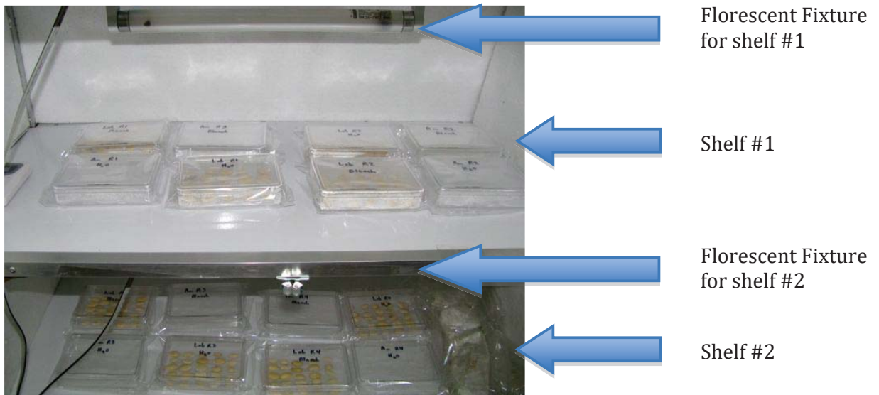
Figure 3: Close-up of 2 shelves used for seed germination, and foam cladding on inside of chamber. A fluorescent tube and ballast hangs from the ceiling of each shelf. Power cords to fluorescent tubes are routed through a hole cut into each shelf into the bottom storage area where the power strip and timer are located.
