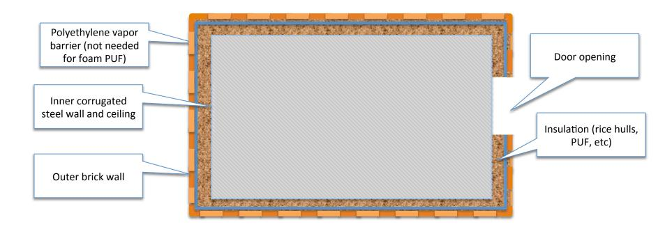
Double wall structure, brick outside, iron sheet (corrugated?) inside. 8' x 8' x 12' Metal roof above ceiling insulation
