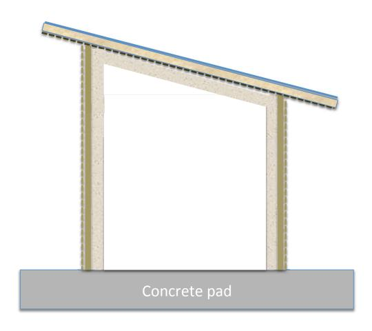
Single wall structure, woven bamboo (?), sprayed PUF insulation
