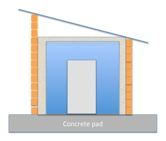
Double wall structure, brick outside, iron sheet (corrugated?) inside. 8' x 8' x 12' Side elevation. Insulation thickness 4 – 12" depending on material. Note vapor barrier around insulation (not needed for PUF)
