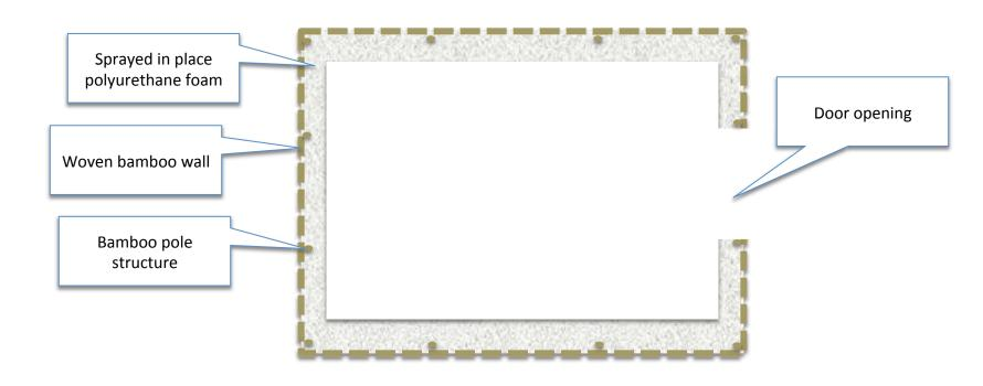
Single wall structure, woven bamboo (?), sprayed PUF insulation  $8' \times 8' \times 12'$  Insulation thickness 4-6 inches. Inside shown, could be outside?
