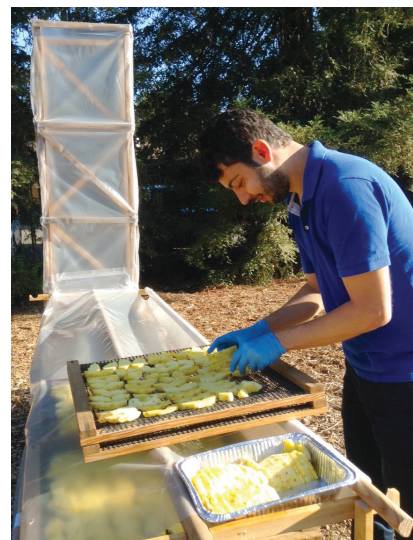
Designed by UC Davis researchers for the Horticulture Innovation Lab, the chimney solar dryer combines solar heat collection with rapid air flow for efficient drying of fresh produce.
